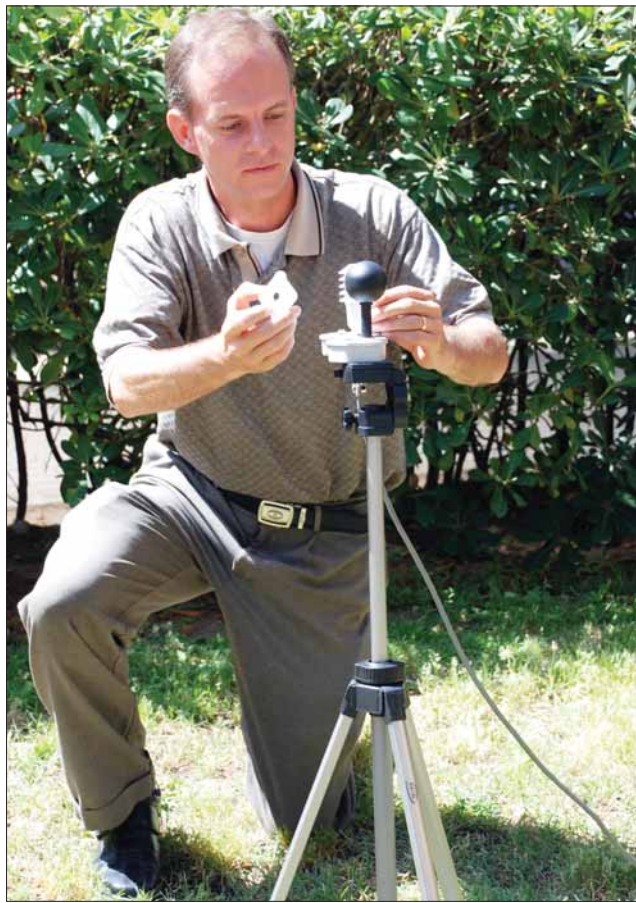
Randy Ross, Safety and Occupational Health manager for USAG Livorno, examines the Wet Bulb Globe Temperature monitoring system on Camp Darby. The system is now linked to the garrison Web site, www.usag.livorno.army.mil , in order to provide instantaneous monitoring to leaders, employees and virtually the entire Camp Darby military community.
